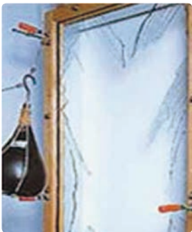
1. Sheet glass(5mm) Very dangerous because of the sharp glass fragments.
