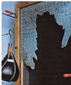
2. Tempered glass(5mm) Shattered, and penetrated by the object.
